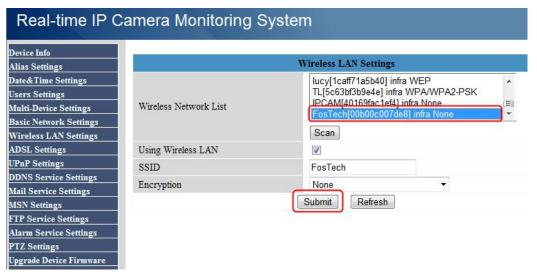
For WEP Encryption , put password in Key1.
