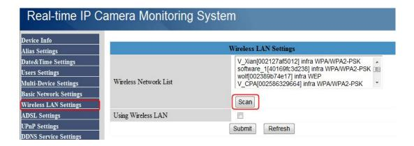
**Step 2:** Click the wireless network which you want to connected. All the parameters would be filled automatically except the password. Put in the password of the wireless network and then click **Submit**.
