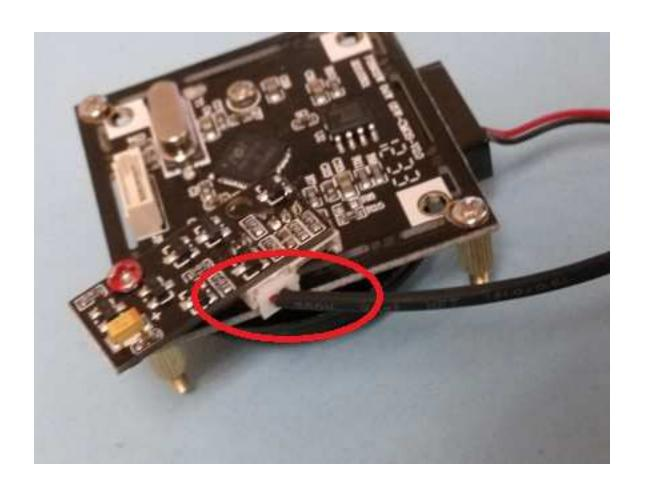
**Connect IR cut-out filter control cable**
