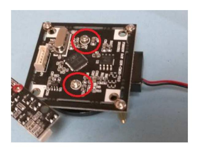
Install 2.8mm IR cut-out filter
