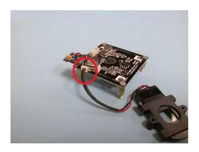
**Disconnect IR cut-out filter control cable**
