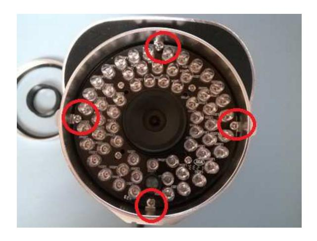
Install LED board / lens assembly retention screws
