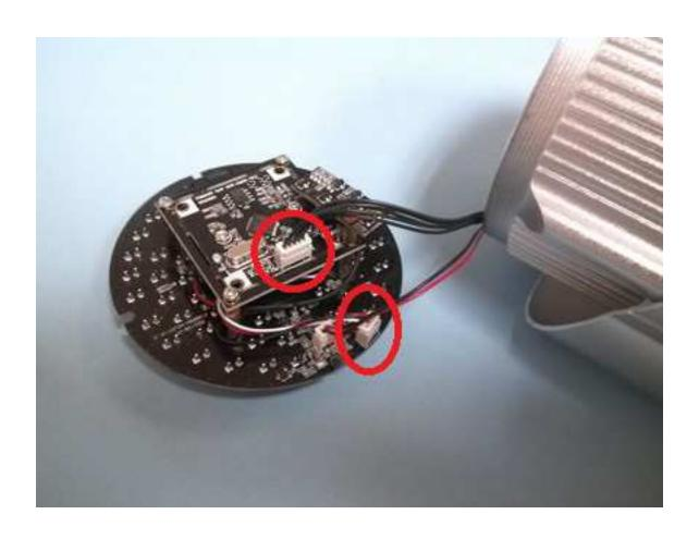
**Connect motherboard interface cable / LED power cable**
