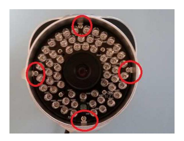
Remove LED board / lens assembly retention screws
