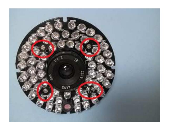
Remove lens assembly retention screws
