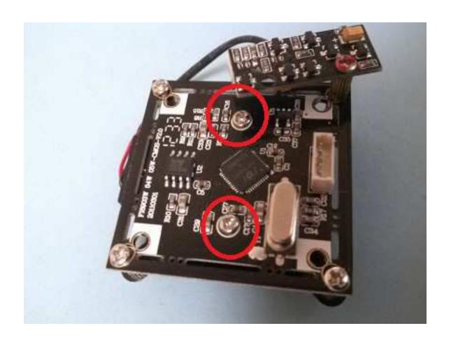
Remove IR cut-out filter retention screws
