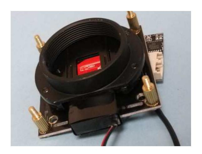
2.8mm IR cut-out filter / lens seat
