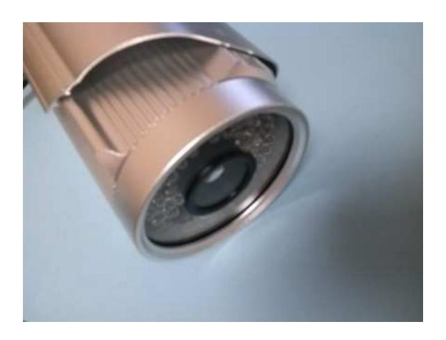
Remove front cap by turning counter-clockwise
