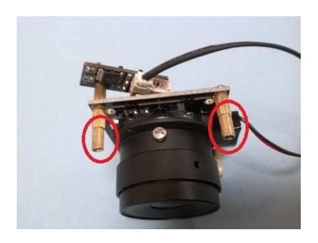
Install short stand-offs, 2.8mm lens, and lens lock screw
