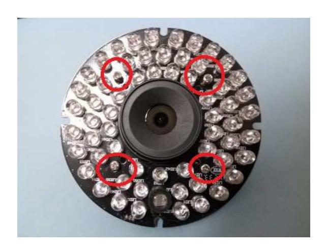
Install lens assembly retention screws
