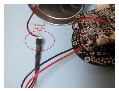
Attach IR Control lead to IR attenuation cable.
