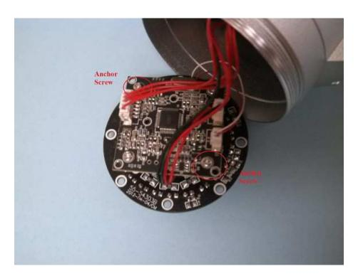
Remove anchor screws securing lens/sensor assembly to IR LED board.
