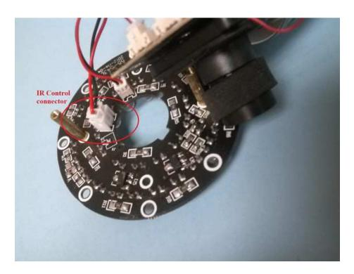
Remove IR Control lead from IR LED board.
