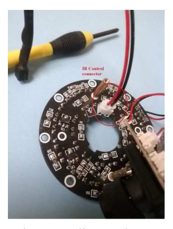
Attach IR attenuation cable to IR Control connector.
