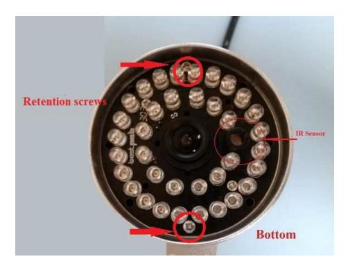
Remove IR LED board retention screws. Make note of the orientation of lens/sensor assembly.
