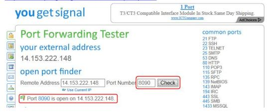
**Step 3:** View camera over Internet by external IP address or host name and port number.
