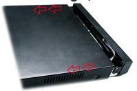
3. Mount the HDD using the 4 screws that came with the NVR, through the base of the chassis:
