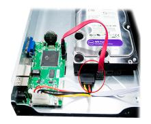
4. Once the HDD has been installed Slide the top cover onto the NVR and re-insert the screws
